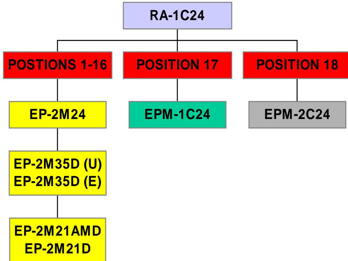
EPB-1C FILLER PANEL SHOULD BE USED IN ALL UNUSED POSITIONS 1-17
