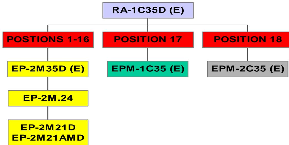
EPB-1C FILLER PANEL SHOULD BE USED IN ALL UNUSED POSITIONS 1-17.
