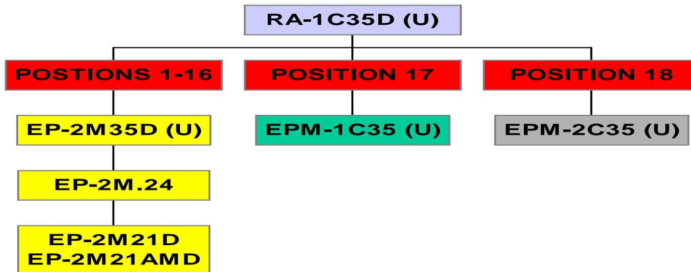
EPB-1C FILLER PANEL SHOULD BE USED IN ALL UNUSED POSITIONS 1-17.
