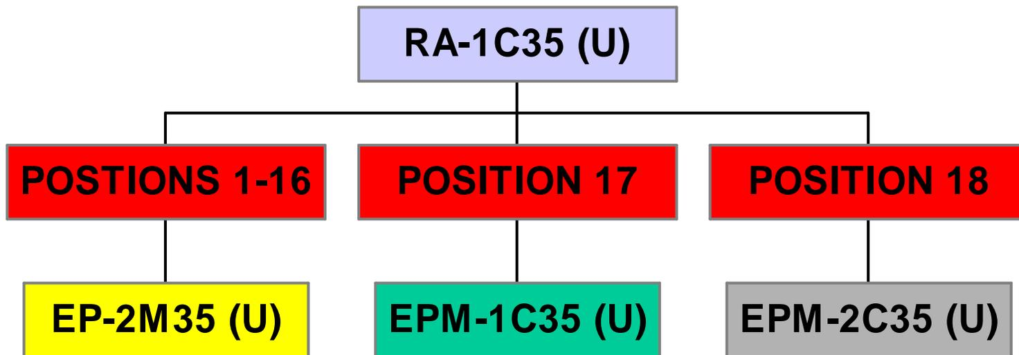
EPB-1C FILLER PANEL SHOULD BE USED IN ALL UNUSED POSITIONS 1-17.
