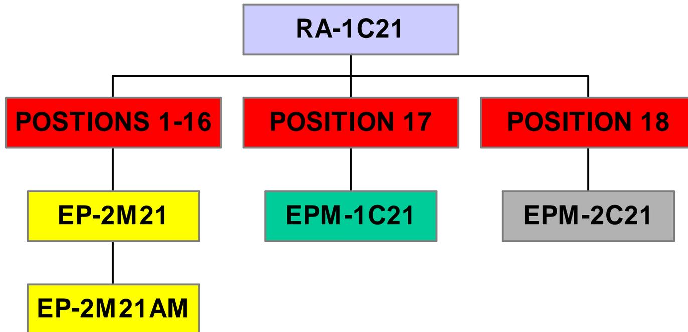
EPB-1C FILLER PANEL SHOULD BE USED IN ALL UNUSED POSITIONS 1-17
